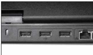
6. Connect one end of the USB cable to the USB port on the back of the S2 and connect the other end to the USB port on the back of the laptop. Each end of the USB cable is designed to fit only in a matching receptacle. The USB cable should connect to the S2 and laptop easily without being forced.
